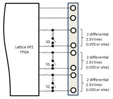
The single-ended wires can be used to connect I2C, SPI or other signals.
