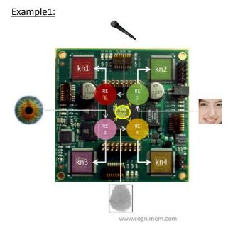
Robust recognition of a person based on its iris and fingerprint and if the person has authorized access to the "appliance" detection of its emotions based on its facial expression and tone of voice.
