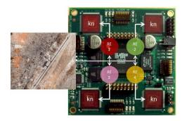
The four quadrants of a high resolution image are recognized in parallel by four neural networks (of 1024 neurons or more) loaded with the same knowledge. The latter can be simple and just intended to recognize edges or simple objects, or it can be more complex and composed of neurons assigned to different contexts to build a decision based on multiple features.
