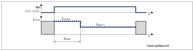
Figure 19 Over Load current thresholds
