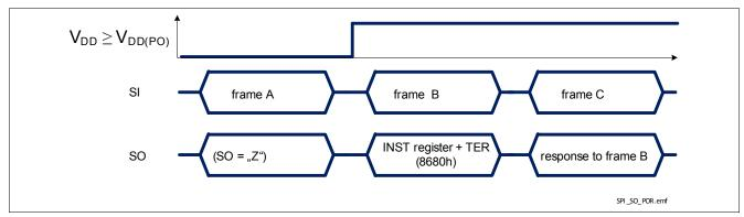
Figure 35 TLE75080-EMH response after coming out of Power-On reset at  $V_{
