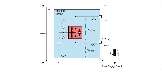
Figure 16 Output Clamp concept
