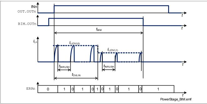
Figure 17 Bulb Inrush Mode (BIM) operation
