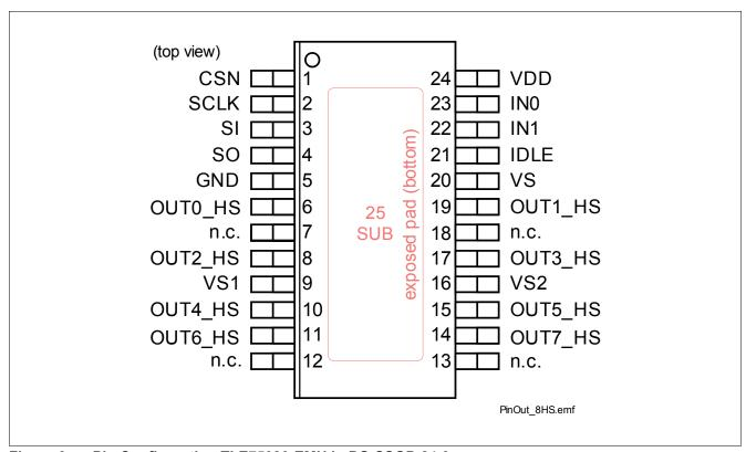
Figure 3 Pin Configuration TLE75080-EMH in PG-SSOP-24-9
