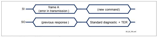
Figure 34 TLE75080-EMH response after a error in transmission
