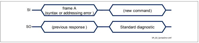
Figure 36 TLE75080-EMH response after a command syntax error
