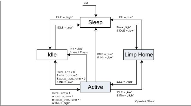
Figure 12 Operation Mode state diagram
