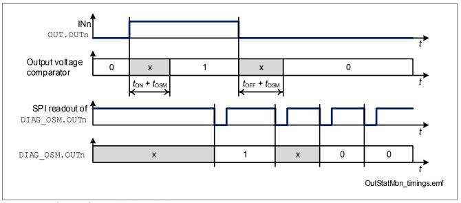
Figure 22 Output Status Monitor timing
