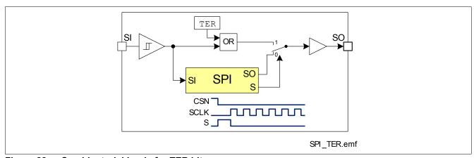
Figure 28 Combinatorial Logic for TER bit
