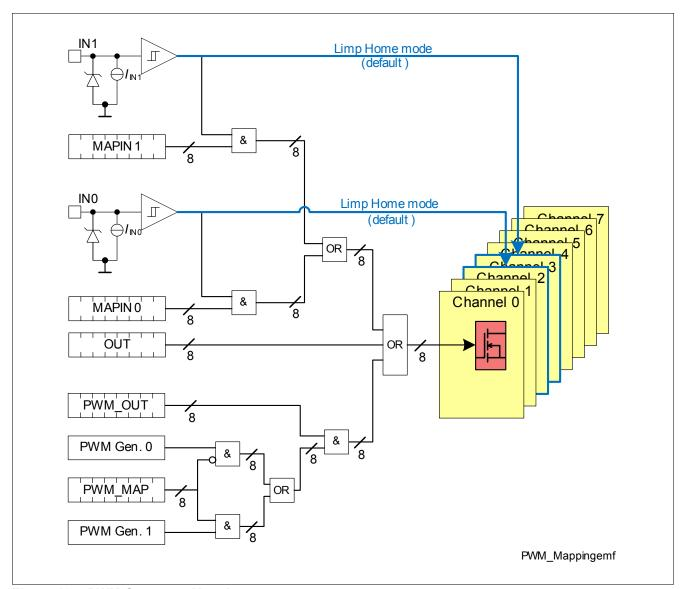
Figure 18 PWM Generator Mappings
