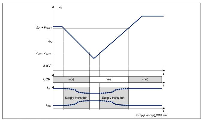
Figure 11 "Cranking Operative Range"
