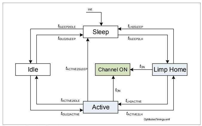
Figure 13 Transition Time diagram
