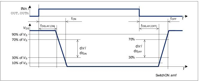
Figure 15 Switching a Resistive Load
