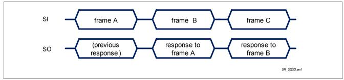
Figure 32 Relationship between SI and SO during SPI communication
