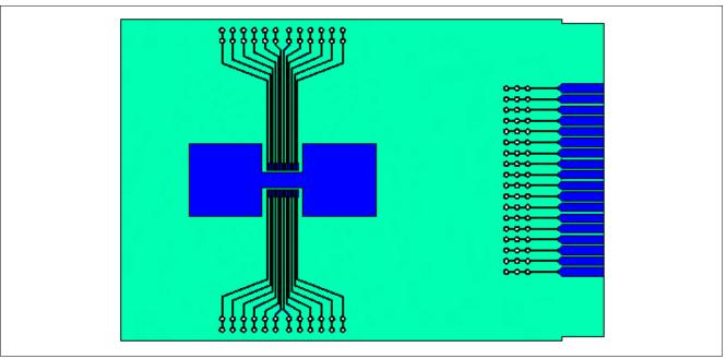
Figure 5 PC Board for Thermal Simulation with 600 mm<sup>2</sup> Cooling Area
