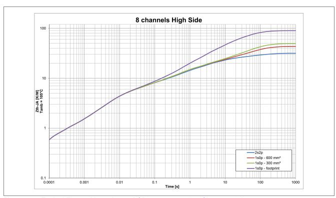
Figure 7 Typical Thermal Impedance. PCB setup according Chapter 4.3.1
