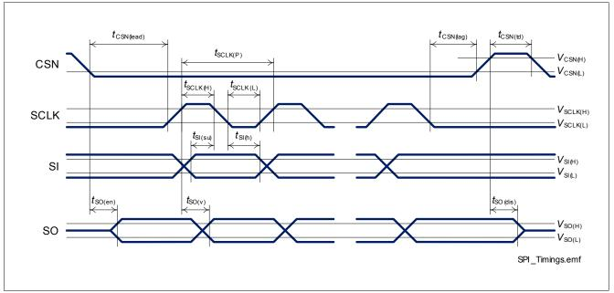
Figure 31 Timing Diagram SPI Access
