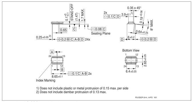
Figure 38 PG-SSOP-24-9 Package drawing
