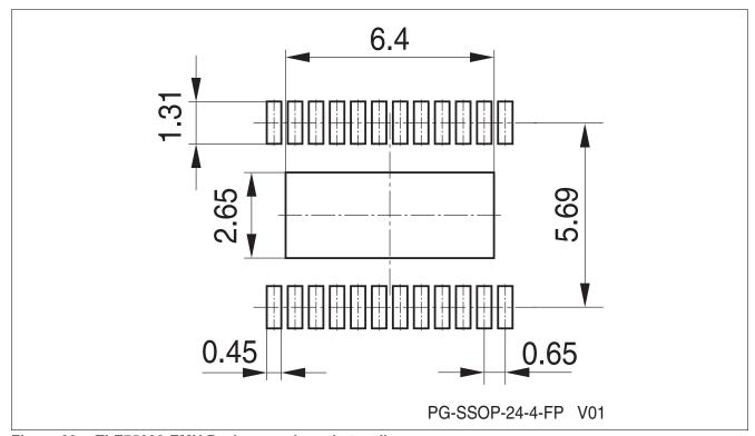
Figure 39 TLE75080-EMH Package pads and stencil
