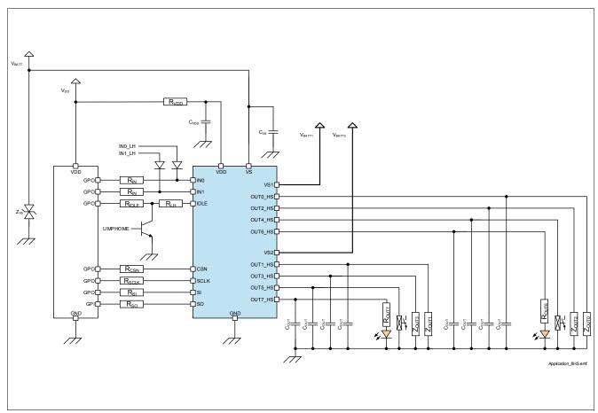
Figure 37 TLE75080-EMH Application Diagram
