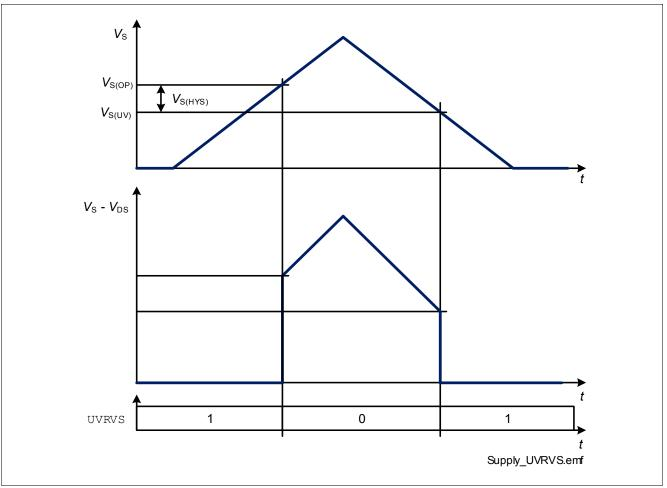
Figure 14  $V_{\rm S}$  Undervoltage Behavior
