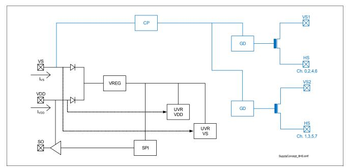
Figure 10 TLE75080-EMH Internal Power Supply concept
