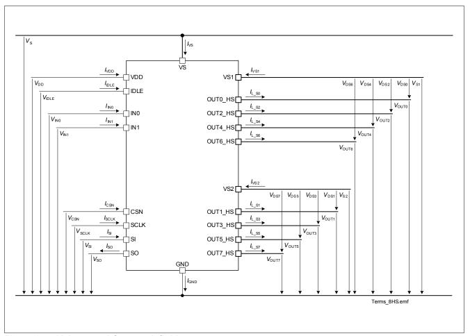
Figure 2 Voltage and Current definition
