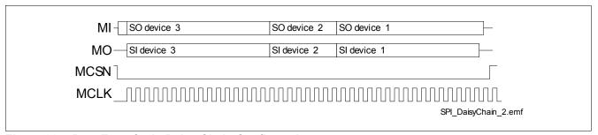
Figure 30 Data Transfer in Daisy Chain Configuration
