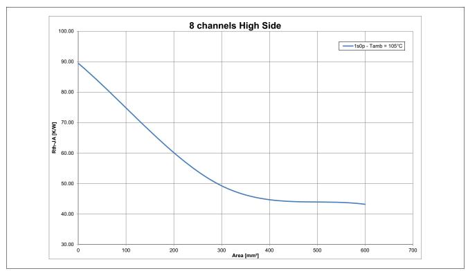
Figure 8 Typical Thermal Resistance. PCB setup 1s0p
