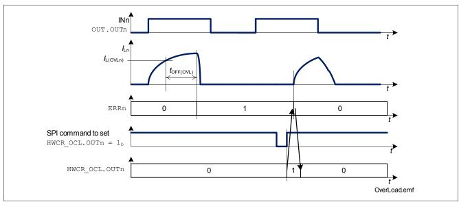
Figure 20 Latch OFF at Over Load
