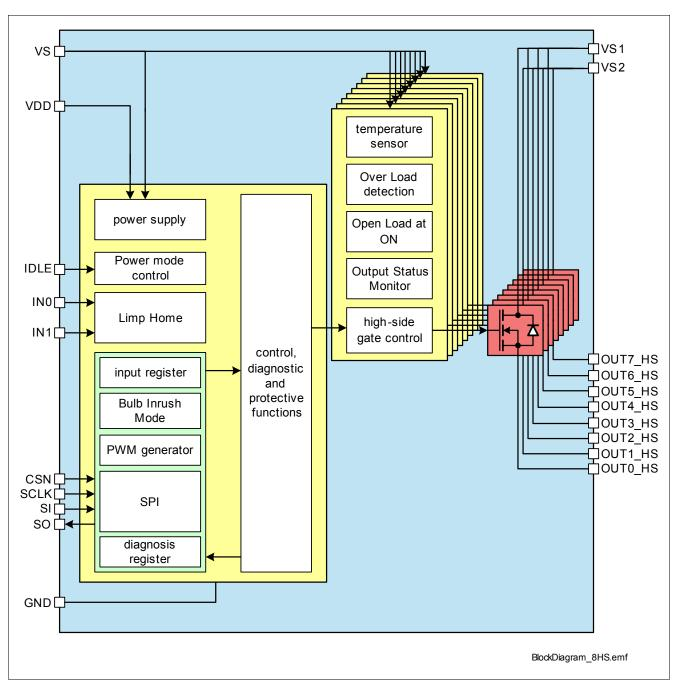
Figure 1 Block Diagram of TLE75080-EMH
