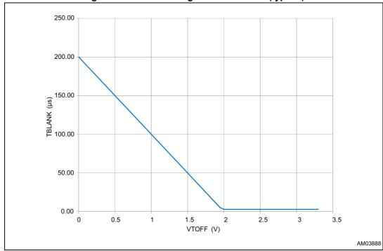
Figure 9. TBLANK voltage vs Tblank time (typical)
