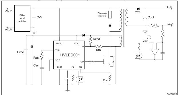
Figure 5. High power factor flyback - constant output current
