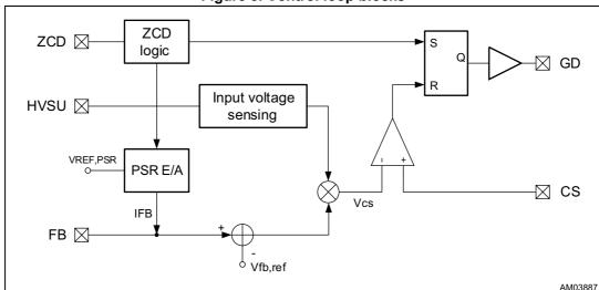
Figure 8. Control loop blocks
