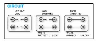
These extra signals are available on the SD connector, but not part of the SD specification, thus they aren't in any specific location manufacturer to manufacturer. Therefore, when designing SD card PCBs you will find that if you change the SD card connector, you will have to redesign the PCB footprint quite a bit.
