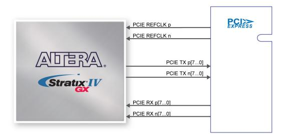
Figure 2–24 PCI Express pin connection
