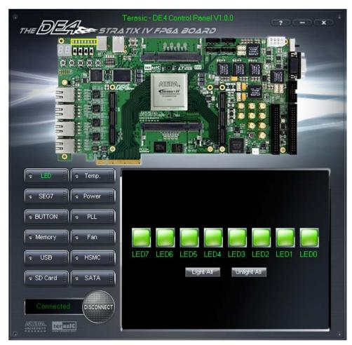
Figure 3–5 Controlling LEDs
