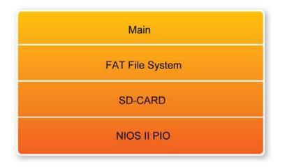
Figure 5–19 Software stack of the SD Card demonstration
