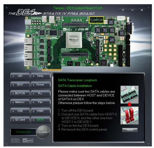
Figure 3–15 SATA loopback verification test performed through the Control Panel
