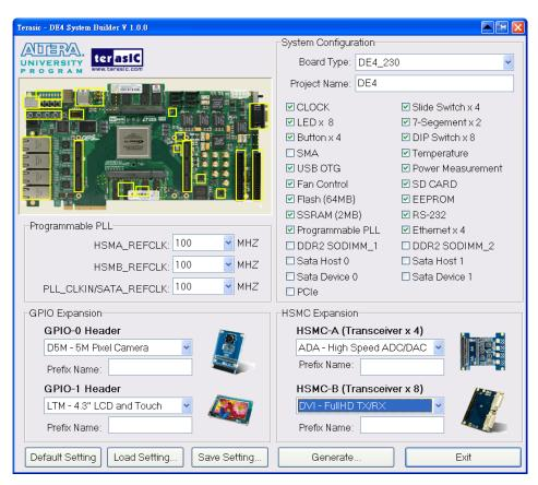
Figure 4–2 The DE4 System Builder window
