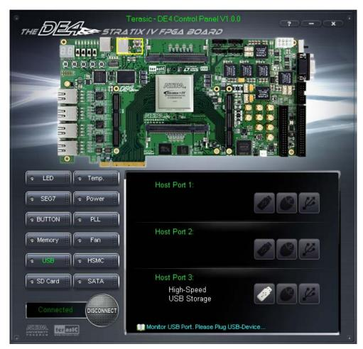
Figure 3–10 Monitoring status of USB ports
