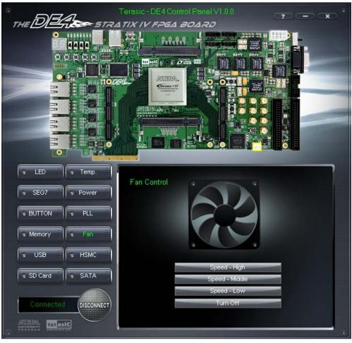
Figure 3–17 Fan Control of the DE4
