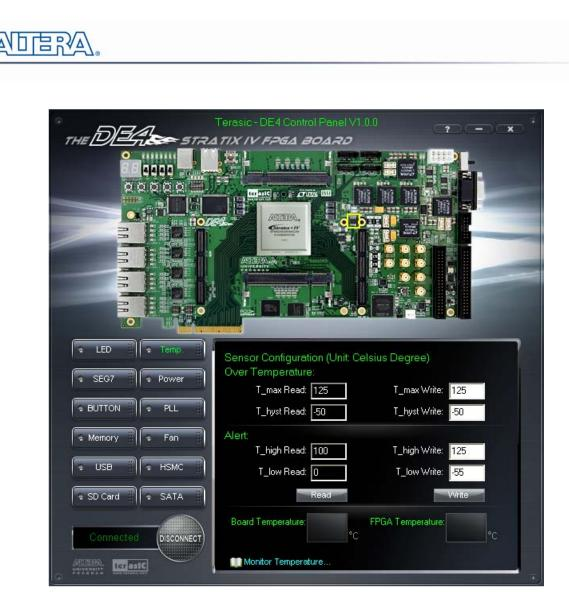
Figure 3–12 Accessing the Temperature Sensor through Control Panel
