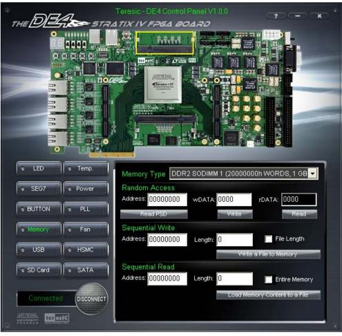
Figure 3–8 Access DDR2 SO-DIMM memory
