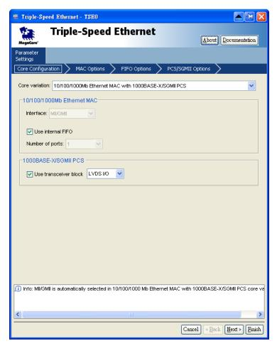
Figure 5–13 Triple-Speed Ethernet core configurations
