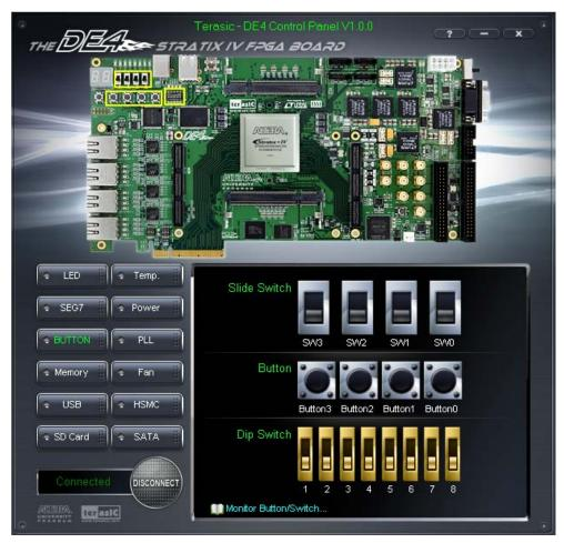
Figure 3–7 Monitoring Switches and Buttons
